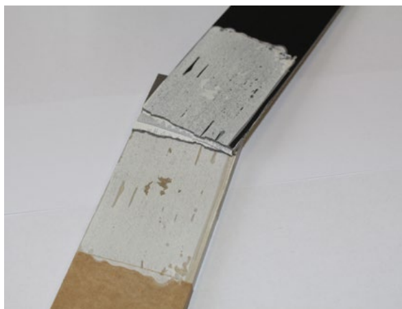
Figure 1 T-Peel sample of an LVT bonded on plywood
